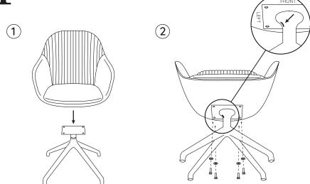
Carefully position the Seat (x1) on top of the Base (x1). Ensure the orientation hole on the base is facing left as shown. Attach the the seat using the Screws (x4) and Washers (x4). Tightly secure using the 5mm Allen Wrench.
