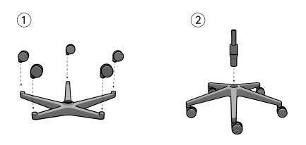
With the 5 Star Base upside-down, push the Casters (x5) into each hole with a fair amount of force (they should 'pop' in). Once completed, turn over so the casters on are on the floor and insert the Cylinder into the 5 Star Base with the larger end on the bottom.
