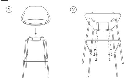
Carefully position the Seat (x1) on top of the Base (x1) and attach using the Screws (x4) and Washers (x4). Make sure the front of the seat is facing the same direction as the footrest. Tightly secure using the Allen Wrench.
